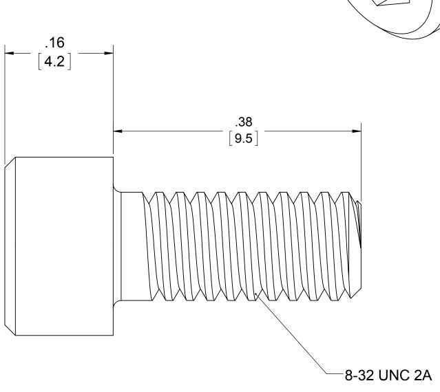
Tolerances: ± 0.02 in / 0.5 mm. All dimensions are in: inches [millimeters]
