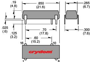
PIN 8: AC LOAD PIN 10: AC LOAD PIN 16: +DC CONTROL PIN 1: -DC CONTROL
