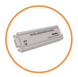
This power management interface module enables a 5V SHG-TT/TS or MHG-TT linear encoder to operate from a 5-28V supply. Output levels remain at TTL 5V quadrature levels.
