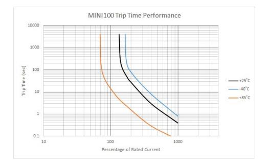
These curves are to be used only as a guide in selecting a protector for a particular application. Final trip times are dependent upon the type of application and are the responsibility of the application engineer to determine through appropriate testing.
