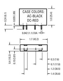
UNLESS OTHERWISE SPECIFIED **DIMENSIONS: INCHES (MILLIMETERS)** TOLERANCE: ±0.020 (±0.50)
