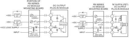
LOAD MAY BE WIRED IN LOCATION A OR B DC INDUCTIVE LOADS MUST BE DIODE SUPPRESSED
