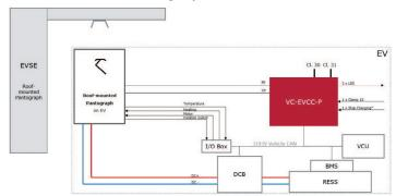
Red components are in focus of EVCC-P system context and are provided by Sensata. Non-red components, e.g. CAN-I/O Interface, have to be supplied alternatively in case Temperature or Heater control shall be implemented.
