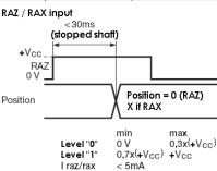
Nota : Do not other connect pinouts, connect DIRECTION and RAZ to a potential (RAZ at OV if not used).
