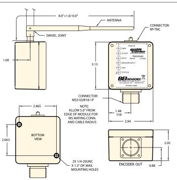
The SwiftComm Receiver Module has an MS connector that provides the same output signals as a standard BEI encoder. Input power can be from 5 to 28 VDC. Quadrature output signals (specified at time of ordering) can be 5 VDC or V in. The B.I.T output signal indicates the RF Link Status. Case ground is internally
