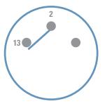
Terminals 1 & 2 are closed and terminals 2 & 3 are open at the high temperature settings
