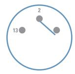
Terminals 1 & 2 are opened and terminals 2 & 3 are closed at the low temperature settings
